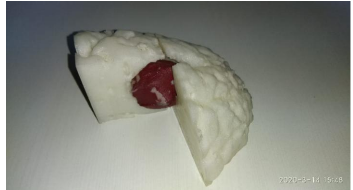
Fig. 17. Final 3D printed cut-section patient specific brain-tumor model
