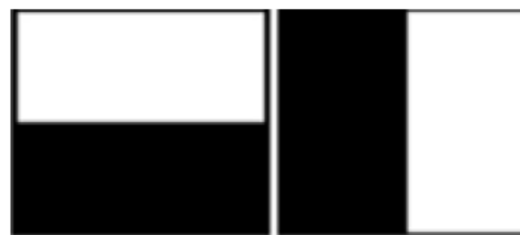
Figure 5.2 Haar wavelet types used for SURF
