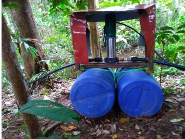
Fig. 10. The 4 HP pump is placed on a wooden structure which is tied to two used chemical drums as floats
