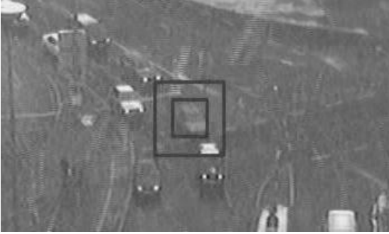
Fig. 2. Center-surrounding approach for modeling the target object and surrounding background. From the inner box foreground (target) object is modeled, while the background is modeled from the outer ring.
