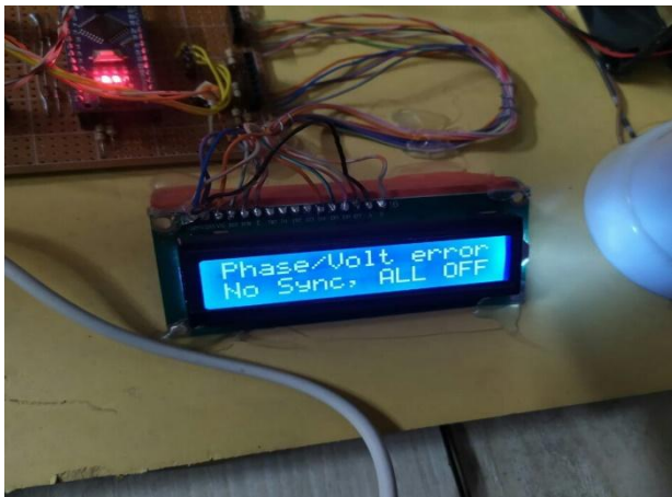
Fig. 14. After take out one phase display show the error and all load has been off
