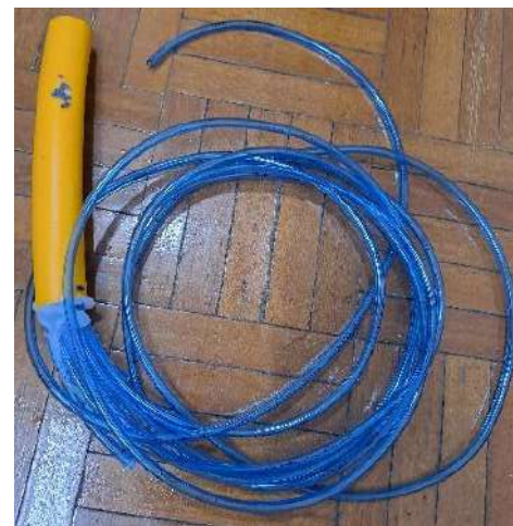
Fig. 22. Initially the outlet hose was forced to send cool air to many tubes, but it did not work
