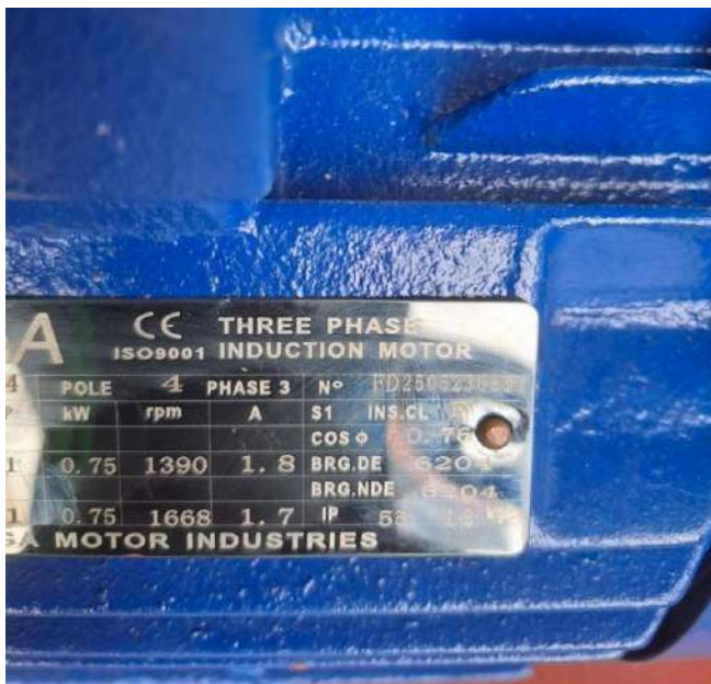
Fig. 6. 3 Φ, 1 HP motor that was subsequently purchased
