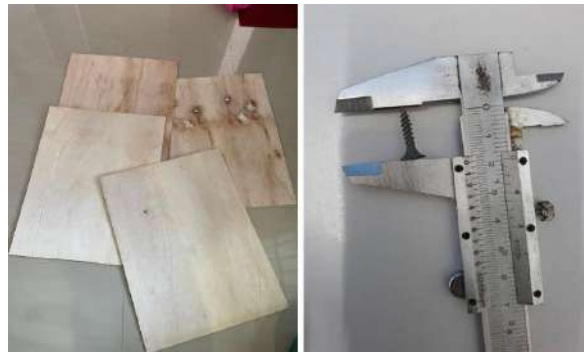
Fig. 8. Four plywood pieces and screw used to join them to form the base of the system; later four wheels were attached to the bottom of the base
