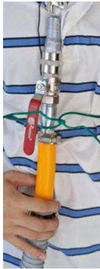
Fig. 18. An air flow valve replaced the VFD in controlling the air flow of cool air out of the system
