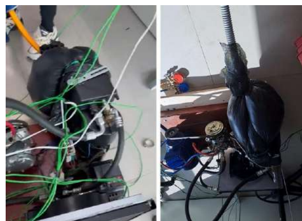
Fig. 17. : Orange hose which was initially used as the outlet and later the flexible and much longer gray hose was used
