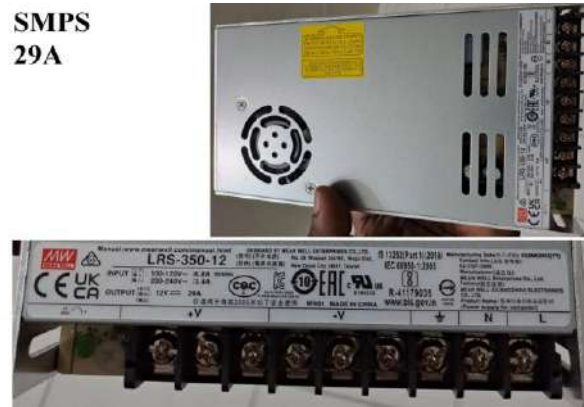
Fig. 7. The 12V SMPS used to power the air-conditioner system but not the induction motor
