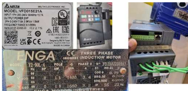
Fig. 12. : The VFD with specs 2HP, 3Φ, below is the nameplate of the 2 HP, 3Φ motor
