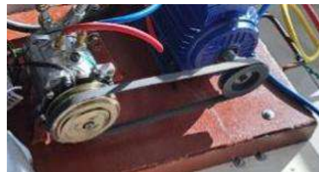
Fig. 9. The metal setup to enable the induction motor to turn the compressor
