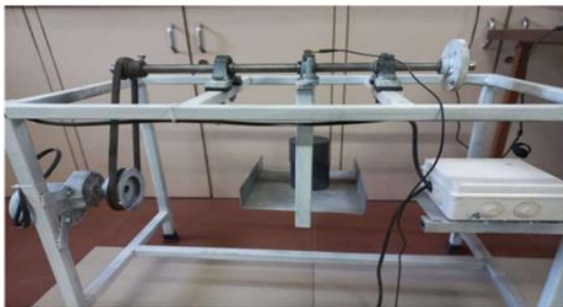
Fig. 1. Experimental setup of fault diagnosis of bearings
