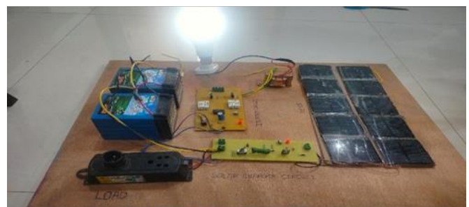
Fig.11 Working operation of solar inverter under load conditions
