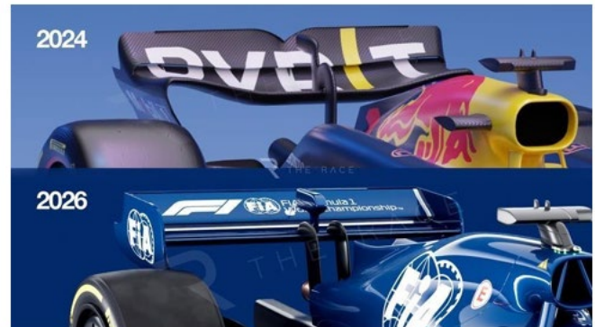
Fig. 14. DRS in 2024 and MOM (Manual Override Mode) according to 2026 regulations
