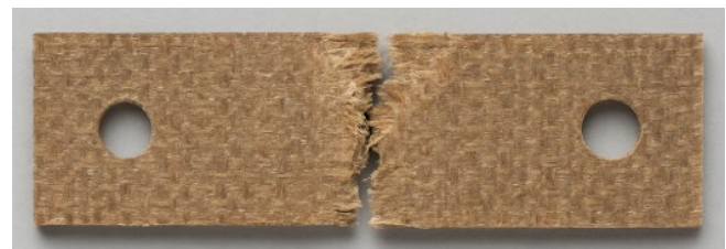
Fig. 7. Reduction in shear-out failures with increasing edge distance.
