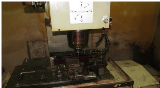
Fig. 2 Drilling process on vertical milling machine
