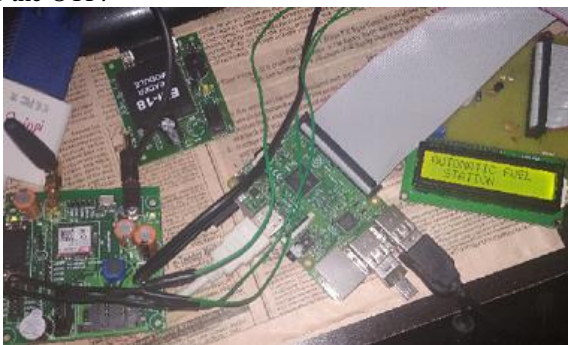
Fig4. Interfacing RFID module with Raspberry Pi
