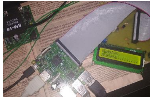
Fig5. Interfacing GSM module with Raspberry Pi
