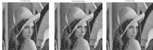
Fig. 3: The decoded LENA image from left to right, (a) original, (b) original OFDM [PSNR= 24.5140 dB], (c) modified OFDM (UEP) [PSNR= 30.4160 dB]
