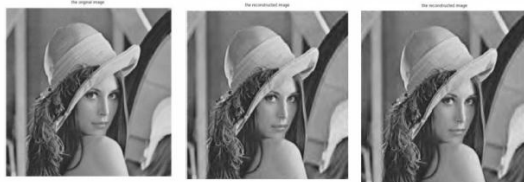
Fig. 5: The decoded LENA image from left to right, (a) original, (b) modified OFDM [PSNR= 30.4160 dB], (c) Modified OFDM with adaptive clipping [PSNR= 29.5970 dB] over AWGN channel at SNR=9 dB with Q BSK
