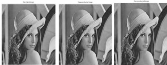
Fig. 7: The decoded LENA image from left to right (a) original (b) modified OFDM [pSNR= 30.4160 dB] (e) Modified OFDM with adaptive clipping [PSNR= 29.9306 dB] over AWGN channel at SNR=15 dB with QAM16
