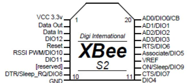
The Operating Voltage for the ZigBee is: 2.1 – 3.6V. The operating Current for ZigBee is 40mA.at 3.3V. Describing about the range, the indoor range is 50 meters whereas the line of sight range is 120 meter. There are 11 digital I/O pins and there are 4 analog I/O pins. RF data rate is 250kbps whereas Throughput speed is 35kbps. Operating range of the Temperature is -40 to 85C.
