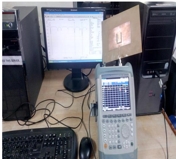
Figure 10: Experimental Setup of antenna testing using Vector Network Analyzer (VNA)
