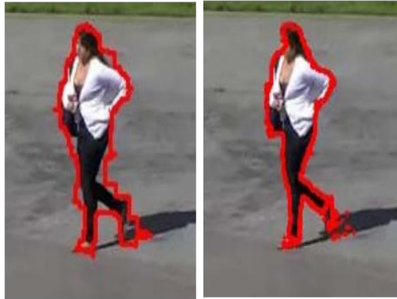
Fig (a) boundary obtained by the moving edge map, (b) boundary obtained by the base mask using color analysis.
