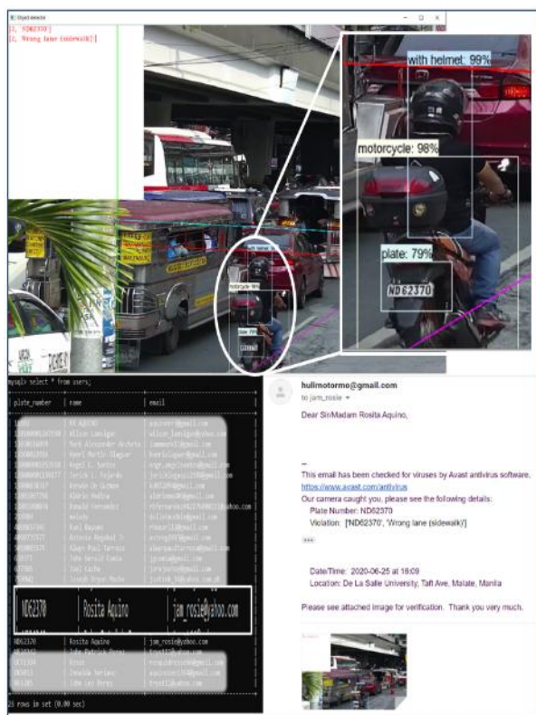
Fig. 9. (a) Sidewalk Violation Detection (b) Plate Detection and Recognition (c) E-mail Notification
