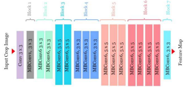
Fig. 3. EfficientNetB0 model with MBCConv blocks for feature extraction.
