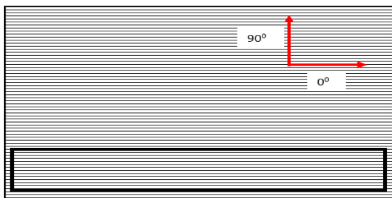
Fig. 5. Schematic of specimen cutting from laminate
