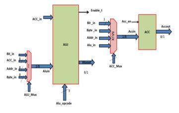
Fig. 3c IL Processor Execution Entity
