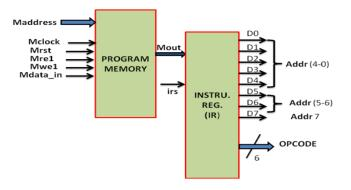
Fig. 3b IL Processor Instruction Decode Entity C. Execution Entity
