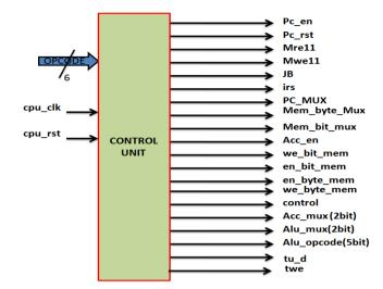
Fig. 3d IL Processor Instruction Control Entity
